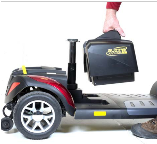
Figure 21. Battery Pack Installation
