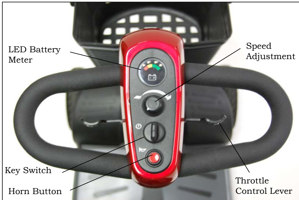
Figure 5. Buzzaround XL™ Delta Tiller Control Panel
