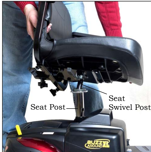
Figure 23. Installing the Seat
